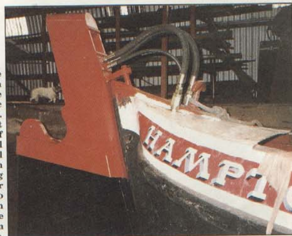
● Detail of the new steel 'ellum showing the hydraulic connections. The upper bracket on the 'ellum is of a non-traditional design with a steel peg, rather than the usual retaining chain. This is for safety reasons so that the 'ellum cannot become detached from its mountings.
