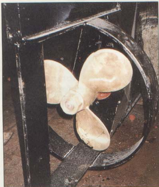
● The steel band is in place and the hydraulic motor is encased in a protective cowling.
